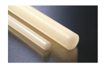
PVDF (polyvinylidene fluoride) is a highly crystalline thermoplastic. Keeps your electrical, thermal and mechanical in a wide temperature range (-40 to 150  $^{\circ}$  C). It is highly resistant to weathering and especially UV rays and Gamma.
